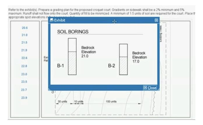
The soil borings exhibit for the croquet court problem. Here bedrock elevations are given relative to topographic elevations. Sometimes soil boring information will be given in depth below the ground surface.
