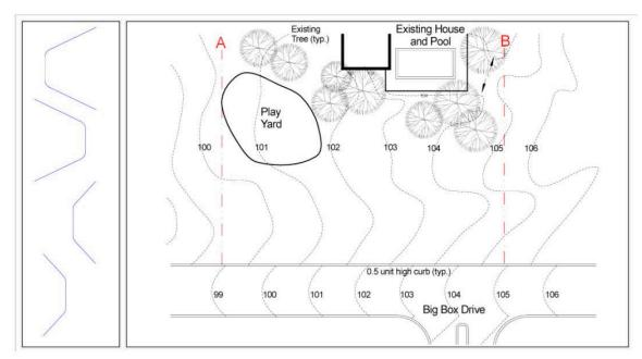
Q. Place the appropriate contours on the site plan to create a 0.5 unit high berm along the existing street between lines A and B. Exhibits
