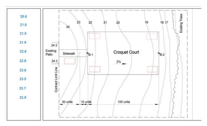
Here the grades are influenced by soils conditions. Here you have a control elevation (ex. Patio), min and max grades on a sidewalk, a directive regarding walk drainage, and criteria for slope and direction of slope on the field. In addition, there are soil borings showing rock depth and a requirement in the problem statement for a minimum of 1.5 units of soil over rock. This is quite a bit more involved than the other AITs we saw earlier.
