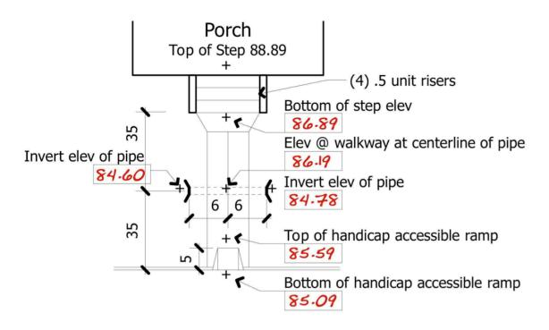
Given: Concrete on walkway .5 units thick, slope 2% .5 unit pipe to slope 1.5% with a minimum of 12" cover over pipe, including walkway
